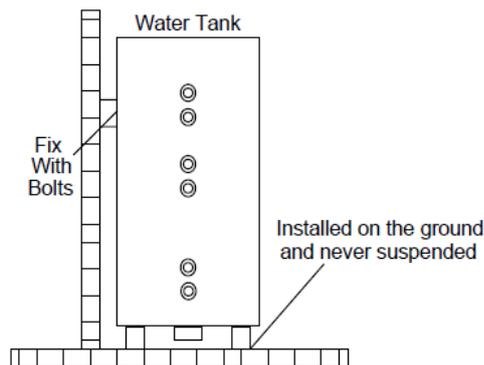
The minimum clearance from the water tank to combustible surface must be 500mm.
