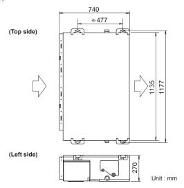
The distance of  $\overset{.}{\times}$  is adjustable according to the place of the hanging bolts. (MAX : 550 mm, MIN : 410 mm)
