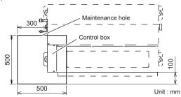
It shall be possible to install and remove the control box, fan units and filter.
