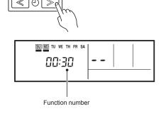
(4) Press the SET TEMP. buttons (  $\vee$  ) (  $\wedge$  ) to select the setting value. The display flashes as shown to the right during setting value selection.
