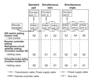
Make sure that the indoor unit with the unit number 00 is connected to the outdoor unit using a transmission cable.
