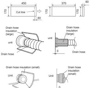
Cover the drain cap with the drain hose insulation.
