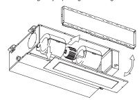
For the bottom air intake, follow the procedure of  $\bigcirc \rightarrow \bigcirc$  for installation. (The factory setting is back air intake.)
