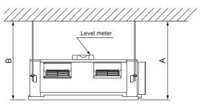
The side A of the unit with the drain port should be slightly lower than the opposite side B of the unit. The height difference between sides A and B should be from 0 to 20mm.
