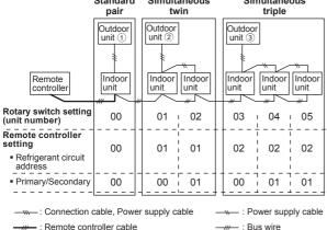
\* Make sure that the indoor unit with the unit number 00 is connected to the outdoor unit using a connection cable.
