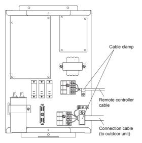
· Do not bundle the remote controller cable, or wire the remote controller cable in parallel, with the indoor unit connection wire (to the outdoor unit) and the power supply cable. It may cause erroneous operation.
