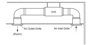
• Be sure to install the air filter in the air inlet. If the air filter is not installed, the heat exchanger may be clogged and its performance may decrease.
