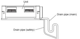
· Once installation is complete, check the flow of the drain water
