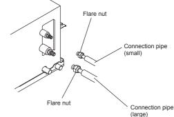
(3) When the flare nut is tightened properly by your hand, hold the body side coupling with a separate spanner, then tighten with a torque wrench. (See the table below for the flare nut tightening torques.)
