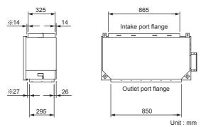
$\%\, {\rm Spacing}$  between flange and drain pan.
