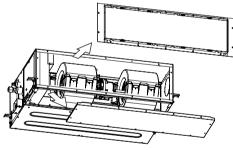
For the bottom air intake, position (1) the intake grille, and (2) the service panel, as shown in the following figure. (The factory setting is back air intake.)
