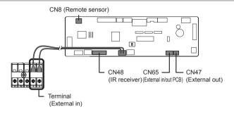
This air conditioner can be connected with the following optional kits. For details on how to install optional parts, refer to the installation manual included in each
