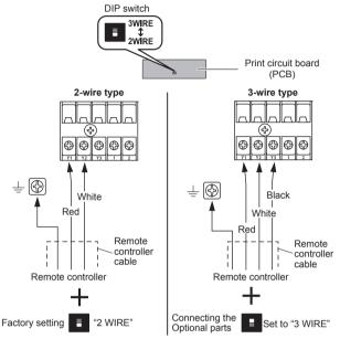
\*Earth (Ground) the remote controller if it has a earth (ground) wire.
