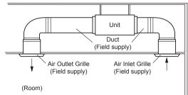
When connecting the duct, perform duct-insulation appropriate for the installing environment.
